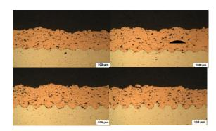
Improving coating adherence thanks to laser texturing (x2)
