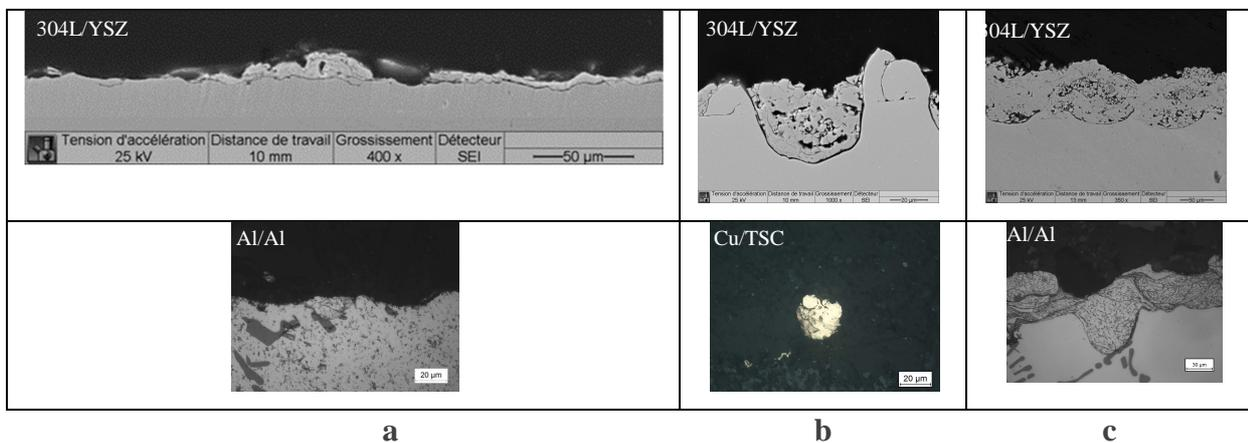
Fig. 4: Microphotographies of interfaces after Tensile Test for Grit-Blasted Surface (a) and textured surfaces: adhesive (b) and cohesive failures (c)
