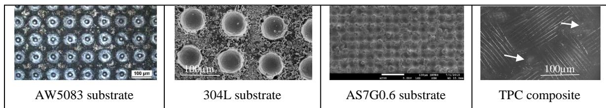
Fig. 1: Example top Views for Al alloys, AISI and composite surface patterning
