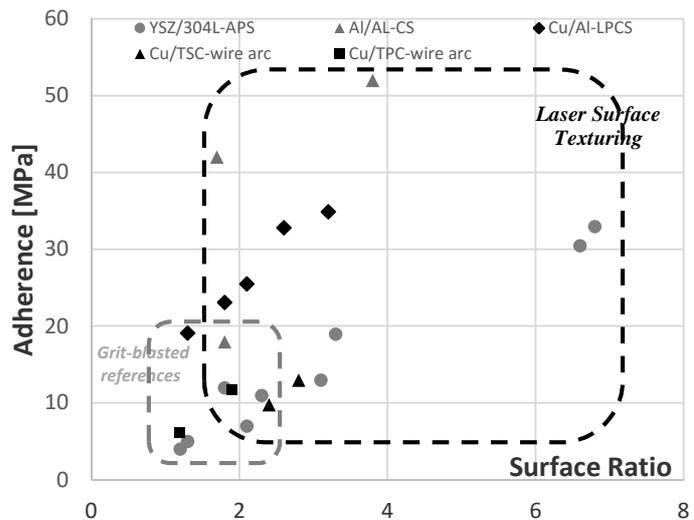
Fig. 3: Coating adherence related to surface ratio considering several material couples sprayed by various processes (grit-blasted references noted by circle).
